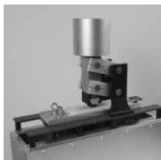
When abraded 1000 cycles by 11 kg (25-lb.) weighted wire brush in laboratory test, IMPERIAL Brand Veneer Plaster Finish showed virtually no penetration—proof of outstanding abrasion resistance.
