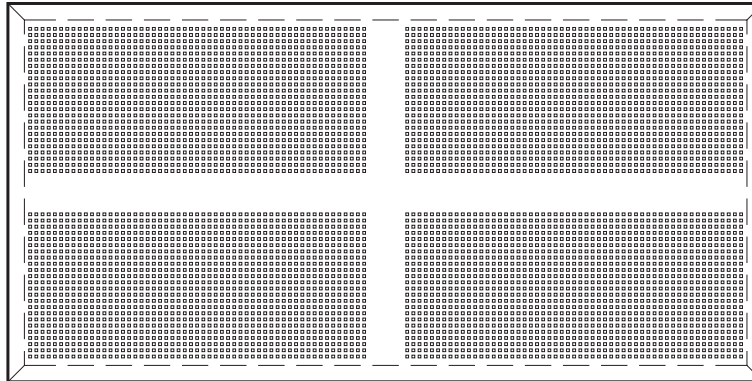
S9 PERFORATION 2L2 PATTERN 4' X 8' PANEL
