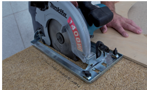
Circular saw: Lay the acoustic panel down with the exposed side down. Always work with a guide and an extraction system. Support the free end of the panel.
