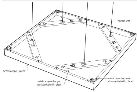
Note: USG Celebration™ canopies are shipped with the hanger brackets and panel closure brackets assembled and attached.
